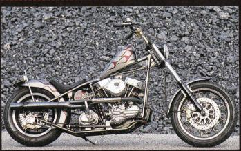
The concept for this machine was to create a good-looking chopper that could handle long-distance touring smoothly and with no stress. This was achieved using an Accurate Panhead engine, a Santee frame and 43mm Ceriani mid-glide forks. With an S&S "G" carburetor and Thunder headers to handle the breathing, this bike boasts high performance while retaining old-school looks through exterior trim and form.
