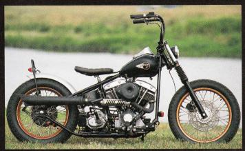
This masterpiece was built with the objective of creating something that nobody thought could exist. With 2" stretch and the neck pulled back 3°, the rigid frame has a custom-built tank created from a 5 gallon Fatbob. It has a suicide clutch and a skull end to the gear lever. It is a unique bike that does not rebel against the latest fashions, but simultaneously does not allow itself to be dictated to by them.
