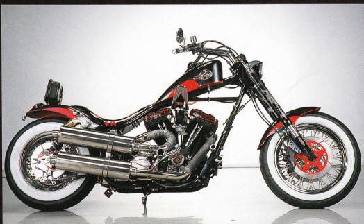
An "Adult Chopper" that was built with no thought of fashion, cost or legality. The rear wheel has 80 spokes for rigidity and carries a Maxis 15-200 tire. The rocker covers have been painted with cracking paint. A Kenny Boyce stretched frame is matched with Ceriani upside-down forks, which have been engraved with a motif of dragons by one of Japan's top engravers.
