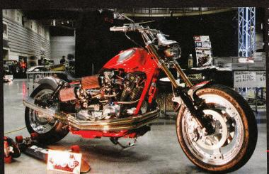
This chopper was built by Sundance for Makoto Watanabe, the editor-in-chief of Hardcore Chopper Magazine. It is a monster machine that uses Dyna's TC88 ignition and is designed for speed. It is the first time that Super XR heads have been fitted on a Twin Cam engine and it represents the peak of Sundance's expertise. Its name is Tequila Sunrise.
