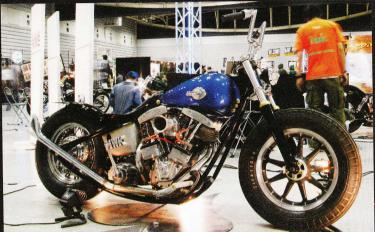
Great care was taken when building this bike to ensure that none of the parts extended beyond the lines of this custom frame. The triple tree was machined out of solid steel. There are lots of amusing touches in its construction from the engraving of a spade on the neck to the headlight bracket, the shape of the tail light, etc.
