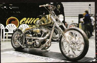
Look at the metalwork on this '94 FXSTC based chopper by Jean in Yamanashi. The tank, seat base and fenders are not gold plated, rather they are made from expensive and difficult-to-work brass. The finish of the unpainted custom parts is typical of Jene Chopper's work.
