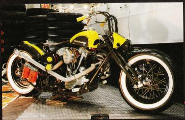
The "Yellow Anniversary 66" was built from a '39 basket case. I boasts new framework that differs from a gooseneck but creates a low profile. It shows numerous unique ideas, such as the fat tank which was converted from one belonging to a Monkey bike, while an extra-large oil filter allows the bike to carry more oil.
