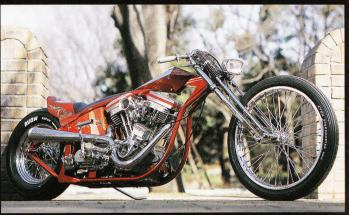
This bike uses aluminum billet parts wherever possible and is fitted with a SuperTrapp muffler. Based on a Softail frame and an evolution engine, it is a seventies-style machine built using twenty-first century technology. The concept behind its design is that of a fusion of digger and drag racer.
